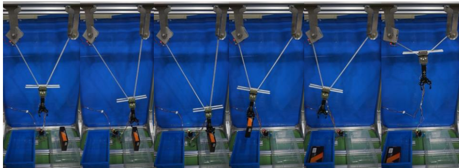
a. deploying b. moving to the right c. grasping d. moving to the left e. releasing f. retracting
