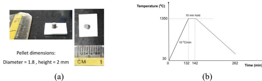
Fig. 1. (a) Sample prepared (b) Heating cycle for High Temperature Microscopy.
