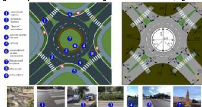
Fig. 5. Design peculiarities of the intersection with circular traffic in the city of Dubno: 1 – pedestrian crossing; 2 – splitter island; 3 – apron; 4 – circulatory roadway; 5 – sidewalk; 6 – landscape design (gardening); 7 – central island; 8 – entry width; 9 – exit width
