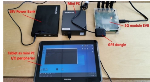
Fig. 3: Hardware used in the implemented testbed setup.
