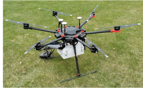
Fig. 4: DJI MATRICE 600 Pro drone with the attached testbed setup.
