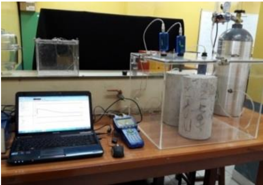
Figure 2. Carbonation chamber and sensors for monitoring the concentration of CO 2 , relative humidity, pressure and temperature inside.
