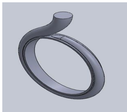
Figure 4: Casing fluid domain part
