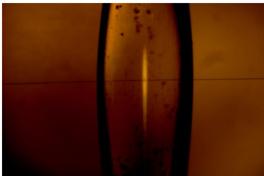
Figure 3. Microscope image of a hollow micro bottle with a maximum diameter of 1354.71 \mu\text{m} and a wall thickness of 94.16 \mu\text{m} traversed by a fiber taper.
