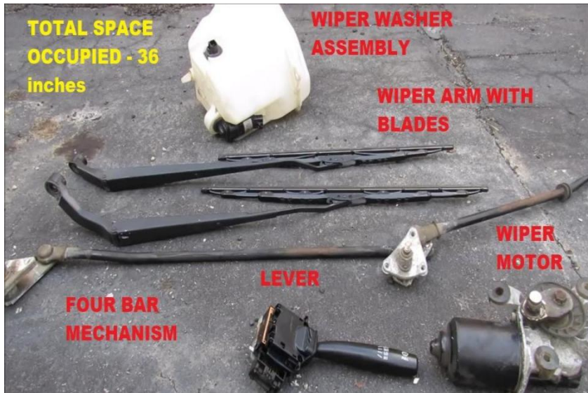
Figure 9 – Various parts of the conventional wiper assembly
