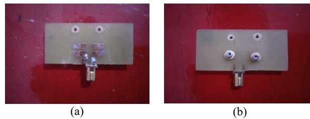
FIGURE 2. Dimensions of the folded dipole microstrip antenna after installing the connector and photodiode: (a) From the front, (b) From the back.
