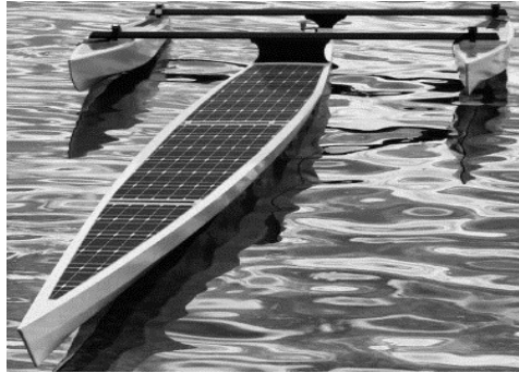
Fig. 1. Prototype of a manned auto embarkation, fed through solar energy
