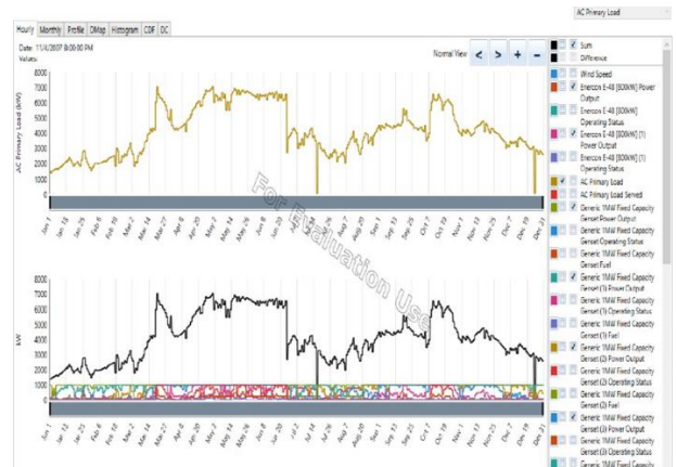
Fig. 7. Comparison of the total power produced by generator (in black) with the total AC load demand (in grey)
