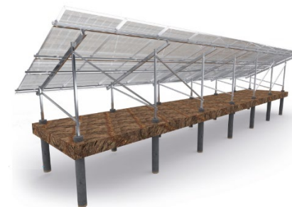
Fig. 4. A Common Structure of Solar Power Station with Use of CONCRETED IN GROUND (BORED PILES)
