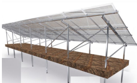
Fig. 2. A Common Structure of Solar Power Station with Use of DRIVIN PILES
