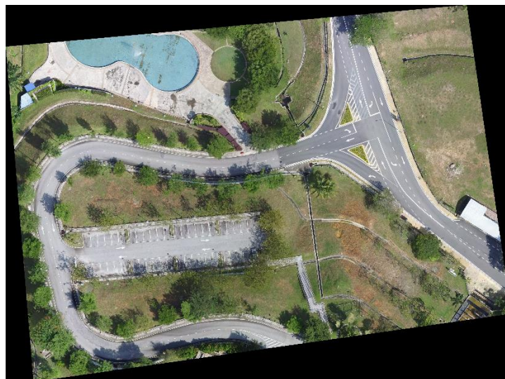
Figure 2. The product of orthophoto generate by Agisoft software
