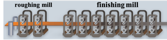
Fig. 3. Schematic diagram of hot rolling manufacturing system.
