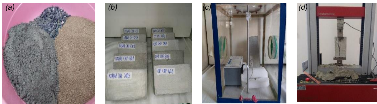
Figure 3: shows (a) mixing of sand, stone and cement (b) fabricated composite brick (c) radon monitor to detect radon gas (d) compression test
