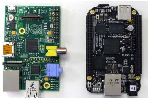
Fig. 7 Raspberry Pi (on the left) and Beagleblone Black
