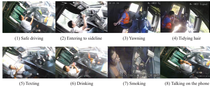
Fig. 2. The Train Drivers dataset contains eight classes, including Category 2 Normal Driving and Category 6 Distracted Driving. (2) in the diagram is normal driving, the thumb and little finger of one hand stand up, indicating that the train enters the sideline. The dataset was recorded by multiple drivers in various environments. The video resolution is 1280 \times 720 at 13Hz.
