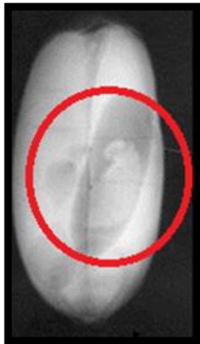
Figure 6 X-ray image of grain and seeds damaged by insect pests of the stock
