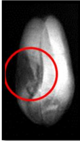
Figure 5 X-ray image of grain and seeds damaged by a bug - harmful turtle
