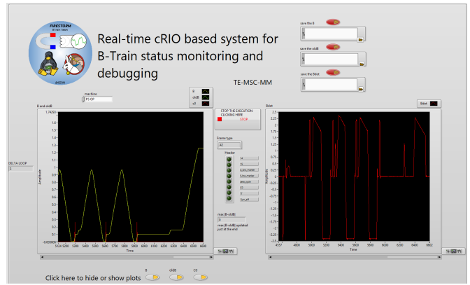
Fig. 4. Front panel of the LabVIEW host user application.
