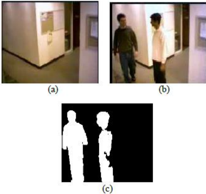
Figure 3: Background subtraction result for hall monitoring video (a) Background model (b) Current frame #89 (c) Resulting frame.
