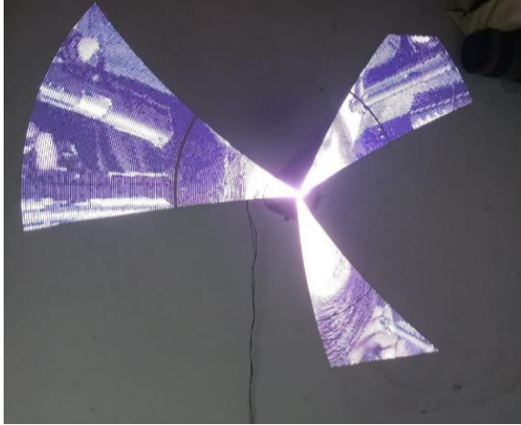
Fig 8 Image of Display when the camera shutter rate not set
