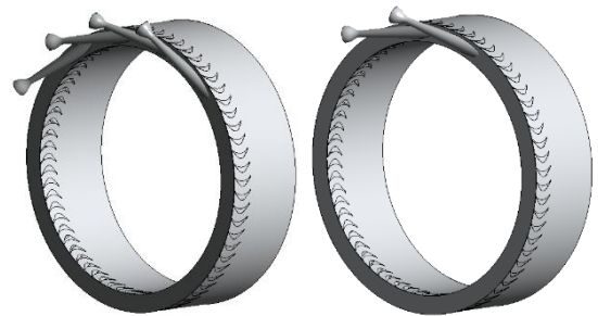
(a) Calculation domain model in the air condition (b) Computational domain model in the underwater condition
