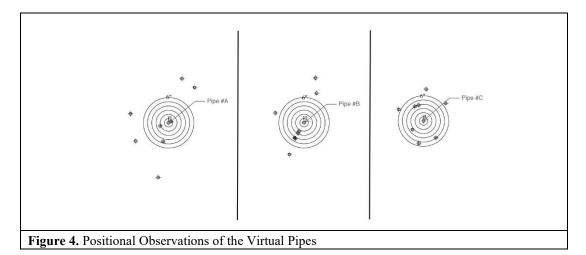
As before, the northing and easting coordinates for each point were measured using a robotic total station and compared to control points to determine placement errors. Table 2 presents the average error distance (in inches), standard deviation, and the quantity of points recorded for each pipe.
