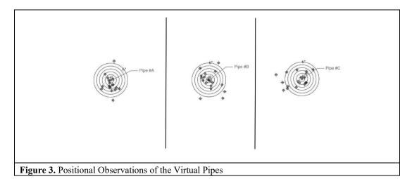
The northing and easting coordinates for each point were measured using a total station and compared to control points to determine placement errors. Table 1 presents the average error distance (in inches), standard deviation, and the quantity of points recorded for each pipe.
