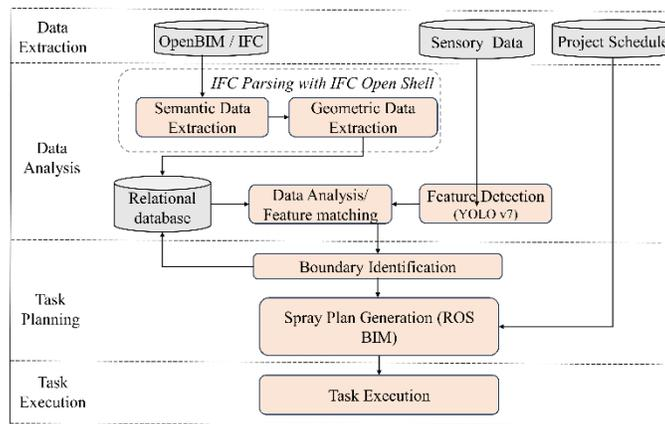
Figure 2. BIM integration framework for autonomous wall painting
