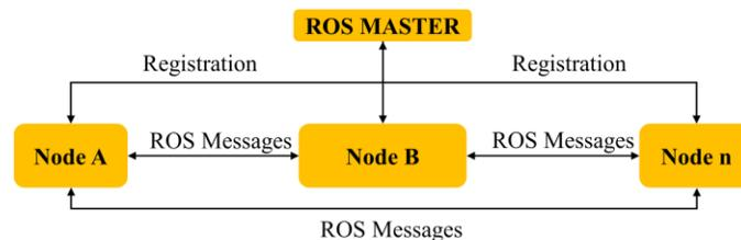
**Figure 6.** Robot Operating System (ROS) operation concept (source: clearoathrobotics.com)
