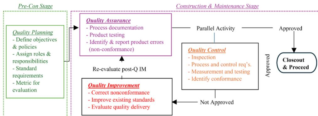
**Figure 1.** Construction Quality Management System Flow Process
